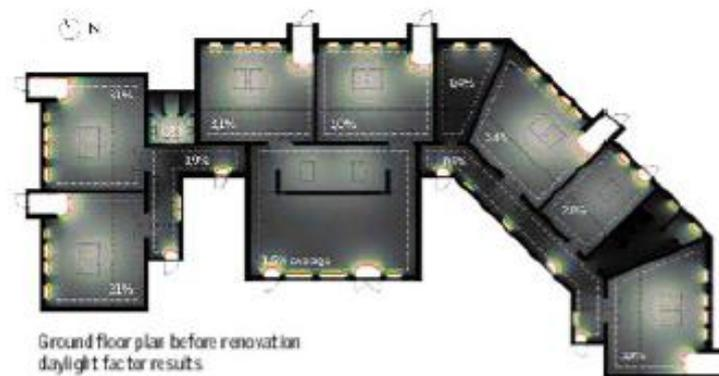
Ground floor plan before renovation daylight factor results
